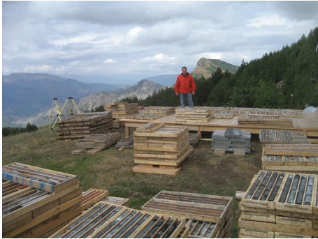
Diamond drill core boxes in storage at the Tirex Resources Mirdita Copper-Gold Property in Albania. Photo courtesy Tirex Resources Ltd.
